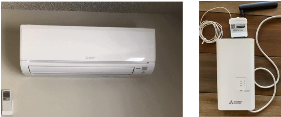
Figure 13: Ecoport/OpenADR communication adapter for Mitsubishi heat pump
